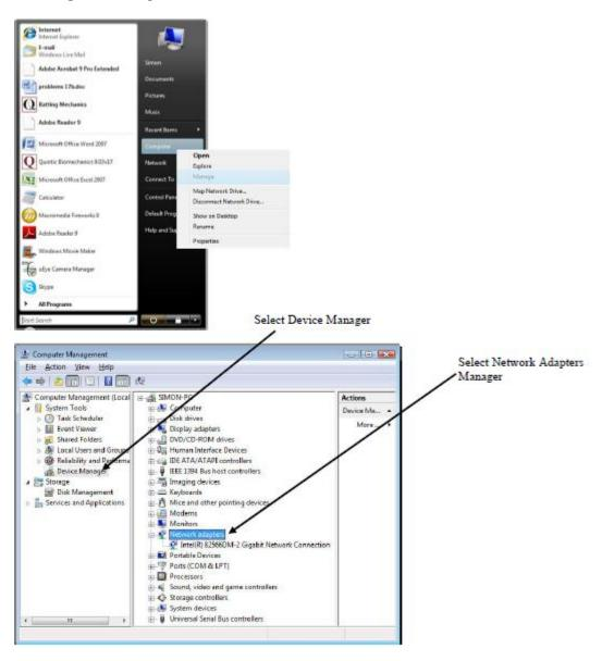
Once you've clicked on network adapters a list of all the network adapters installed on your machine will be shown. To ensure that the GigE camera works at full speed the network adapter must be 100mb or state Gigabit Network connection.
