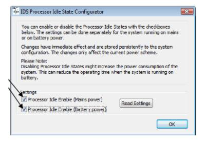
Once the tick boxes have been unchecked, close the window and load up your Quintic Software. Open the live camera feed, you should now be able to record at higher frame rates.
