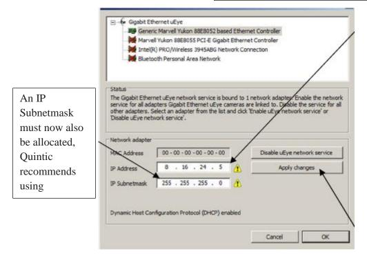
Once an IP address and an IP subnetmask have been allocated click on the 'Apply Changes' button. A window will now appear asking if you wish to assign a static IP address click on 'YES'.
