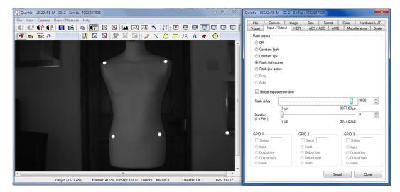
If the camera is already running at it's maximum frame speed, you may need to adjust the size of the image / the area of interest in order to increase the frame speed. The window for this is shown below.
