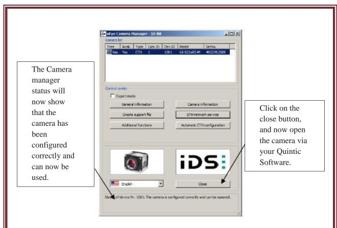
After the ETH configuration is complete, a window may appear asking you to update the firmware this will take place automatically on opening the camera through Quintic. After the Firmware update is completed, please reopen the Camera Manager and select 'Automatic ETH configuration' again.
